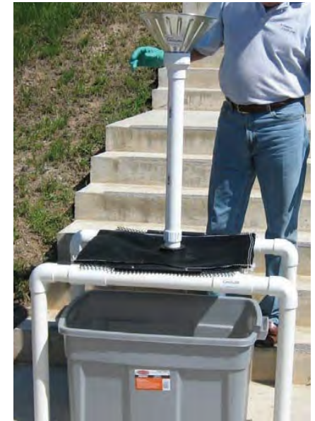
Geotextile Tube Demonstration Test (GDT) (PGDT)
