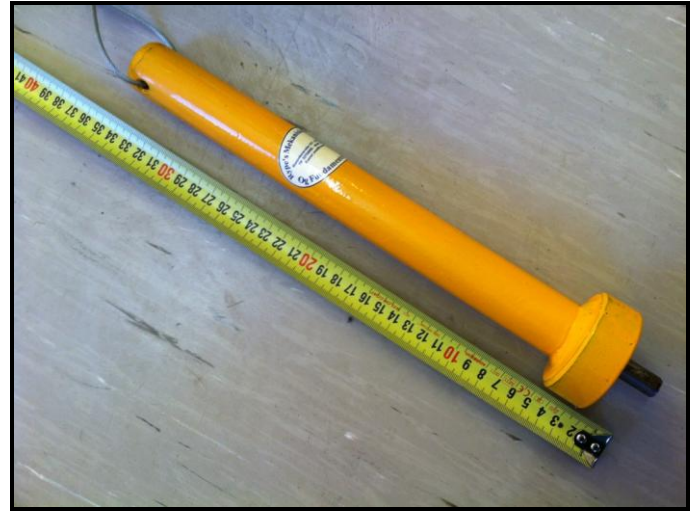
Fig. 11. A hard rock tester similar to the design used on the OMP project.
