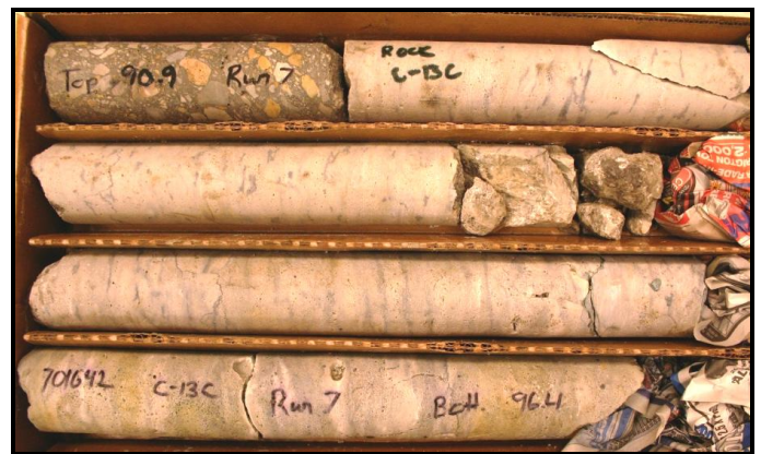
Fig. 14. Bottom of concrete core at Caisson 13 showing clean contact between concrete and dolomite bedrock at 91.8 ft.
