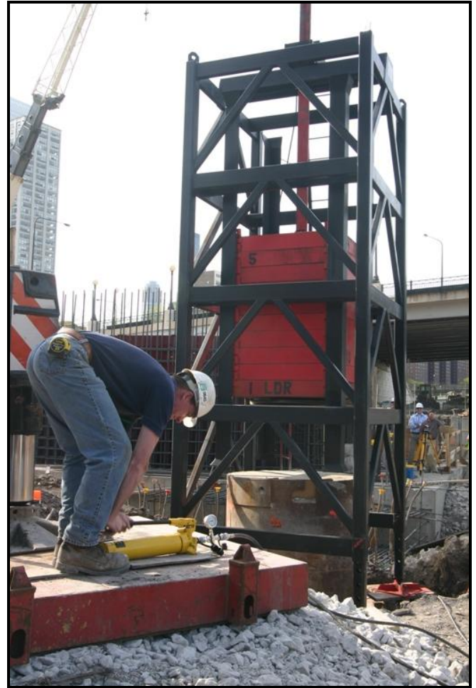
Fig. 20. Forty-ton weight about to be dropped on Caisson 79 to perform a 4000 ton dynamic load test.
