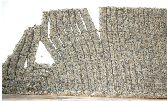
Figure 12(a)(left) - Initial cut-slope, in a block-jointed rock mass with one set dipping steeply into the hillside. 12(b)(right) - Buckling initiated by toppling of this slope.
