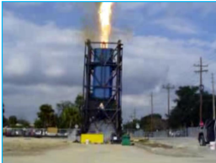
Statnamic Load Test www.statnamiceurope.com
